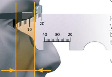
Hold the Personalization Key horizontally, aligning the Vertex Distance Scale with the wearer's cornea. Measure between the cornea and the back side of the lens for the vertex distance.
