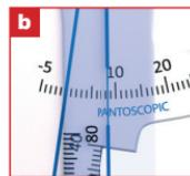
Pantoscopic indicator shows the Pantoscopic angle value on the pantoscopic scale.
